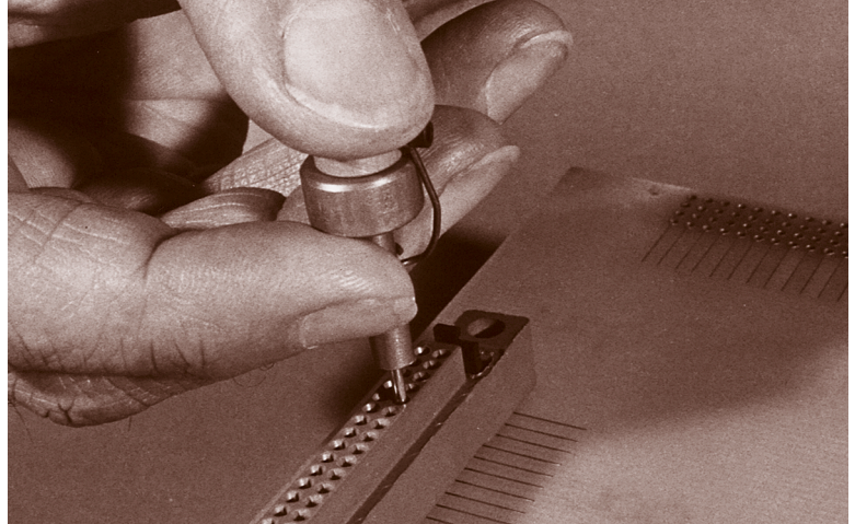
SEAT PLUNGER AND REMOVE CONTACT AND TOOL
