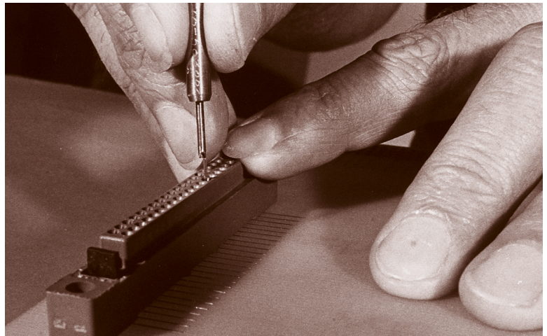
SEAT CONTACT WITH INSERTION TOOL
